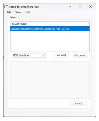
The USB 2.0 interface is provided as a COM port. Multiple connected devices are listed.
