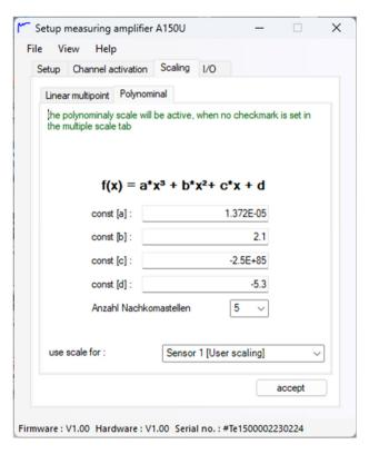
For example, use EXCEL to calculate a polynomial function with 4 constants and enter the values accordingly.
