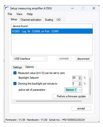
The TFT backlight can be dimmed to a fixed percentage. To do this, select the «Options» tab and change the setpoint.
