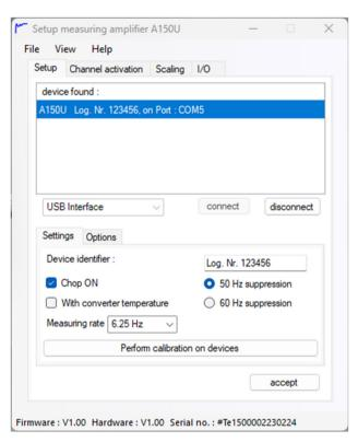
Chop ON: This setting is used to minimise offset drift when the measurement rate is less than 300 Hz.
