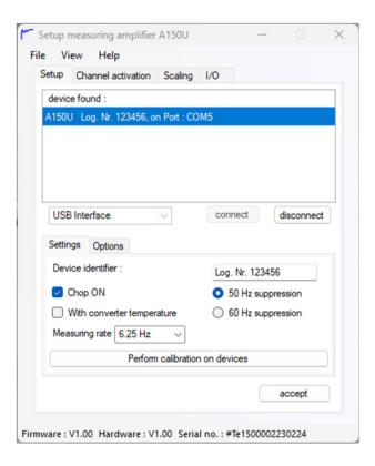
The measuring amplifier does not require sporadic auto-calibration, but internal device calibration can be performed manually.
