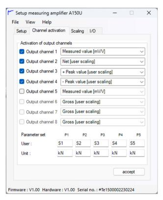
Assign the desired measured values to the output channels. The names of the user parameter sets [CH1...5] can be changed if desired. The display shows, for example, S1 Net. The units are assigned to the parameter set and must be entered accordingly. They are used for user scaling.
